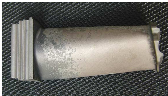
Fig. 6. Sulphidation attack of a turbine blade. Such damage can sometimes be repaired by removing the damaged coating and re-applying a new coating.
