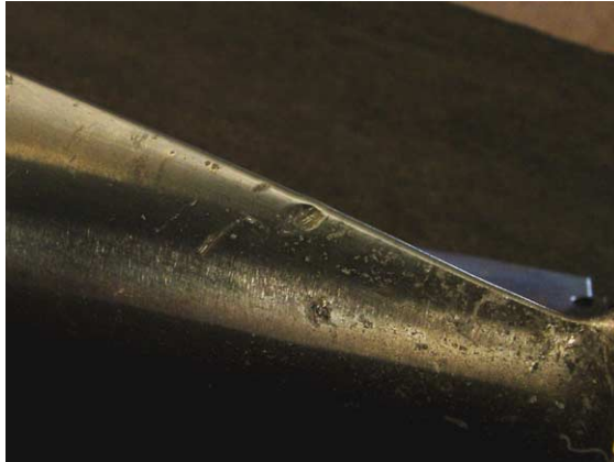
Fig. 2. Mechanical damage caused by ingested foreign material on the leading edge of a compressor blade.
