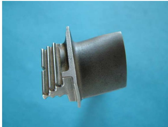
Fig. 1. A typical high pressure gas turbine blade.
