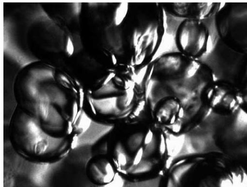
Fig. 1. A microscopic photograph with circa fifteen particles is shown. The dimension of the picture is 1061 \mu\text{m} \times 762 \mu\text{m} . The mean length of the particles evaluated from 10 such photographs is 344 \mu\text{m} and the standard deviation 136 \mu\text{m} . The mean width was determined to be 234 \mu\text{m} and the standard deviation 85 \mu\text{m} . A width to length ratio of 0.68 is therefore, calculated. The effective length was determined by a theoretical model from the projections given on the photographs.
