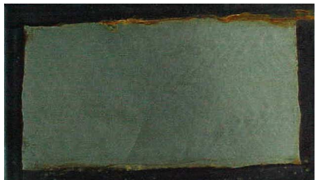
Fig. 16. Salt spray tests results for WC–10Co–4Cr, 150 \mu\text{m} thickness.
