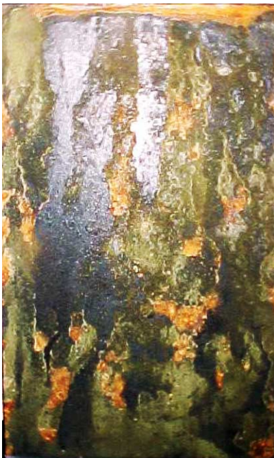
Fig. 14. Salt spray tests results for WC–17%Co HVOF I, 250 \mu\text{m} thickness.
