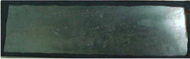
Fig. 17. Salt spray tests results for WC–10Co–4Cr, 200 \mu\text{m} thickness.
