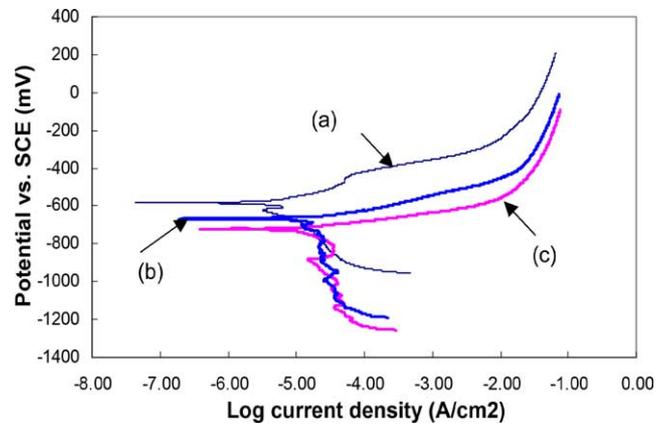
Fig. 8. Potentiodynamic polarization curves of different surfaces in 3.5% NaCl solution: (a) full annealed; (b) Charpy impact fractured; (c) slow bending-fractured.
