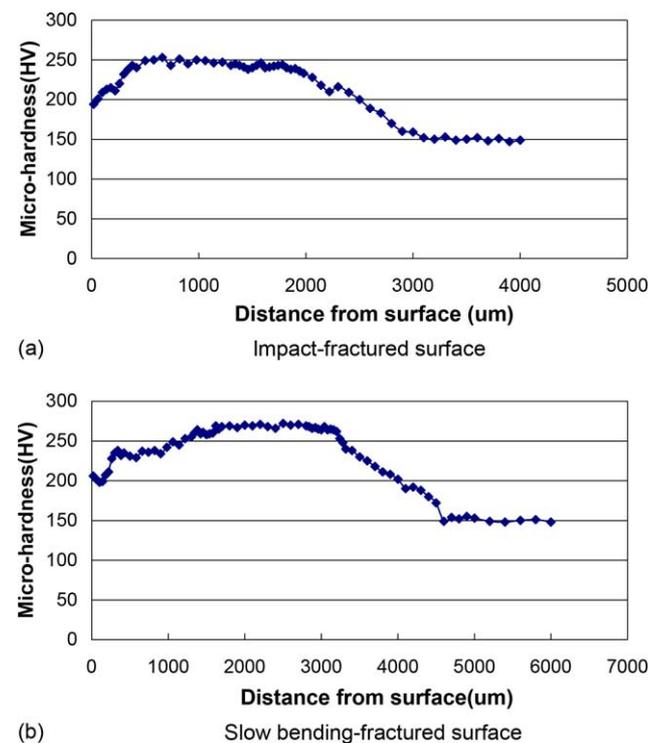
Fig. 6. Micro-hardness of impact-fractured and slow bending-fractured surface layers: (a) impact-fractured surface; (b) slow bending-fractured surface.
