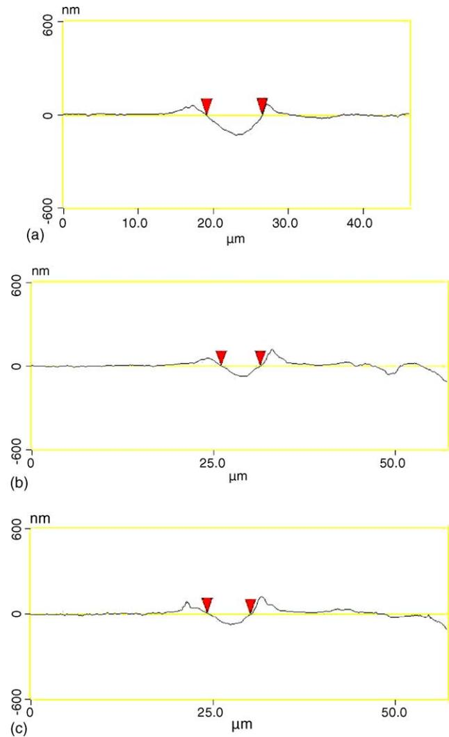
Fig. 10. Cross-sectional profiles of scratch grooves generated by scratch in 3.5% NaCl solution at a load of 5 g: (a) annealed; (b) impact-fractured; and (c) slow bending-fractured.
