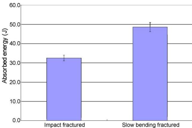
Fig. 4. Absorbed energies of Charpy impact and slow bending tests.
