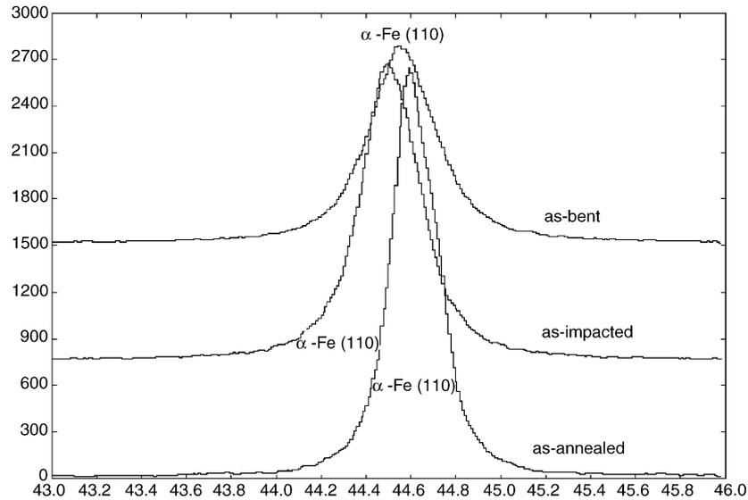
Fig. 7. X-ray (1 1 0) diffractions of full-annealed, impact-fractured and slow bending-fractured surface layers.
