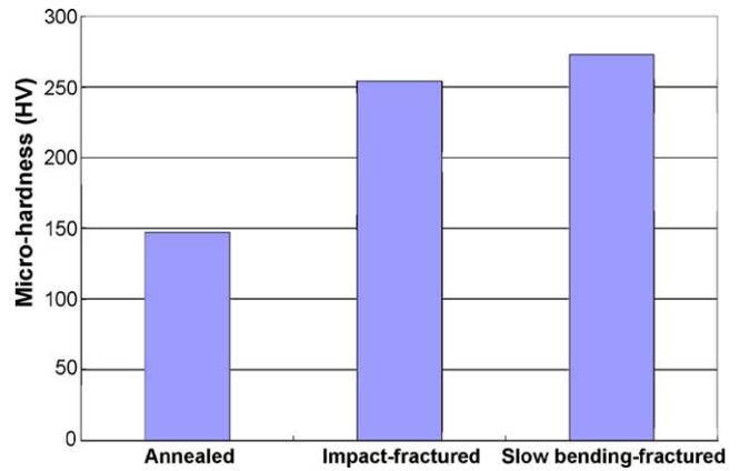
Fig. 5. Micro-hardness of annealed, impact-fractured and slow bending-fractured sample surface.
