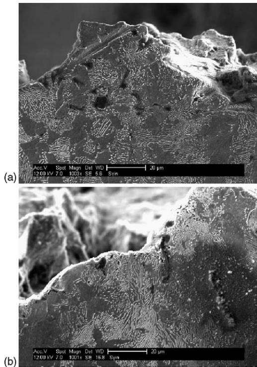
Fig. 3. SEM observation of microcracks in fracture surface layers: (a) microcracks in fracture surface layer caused by the Charpy impact test; (b) microcracks in fracture surface layer caused by slow bending test.
