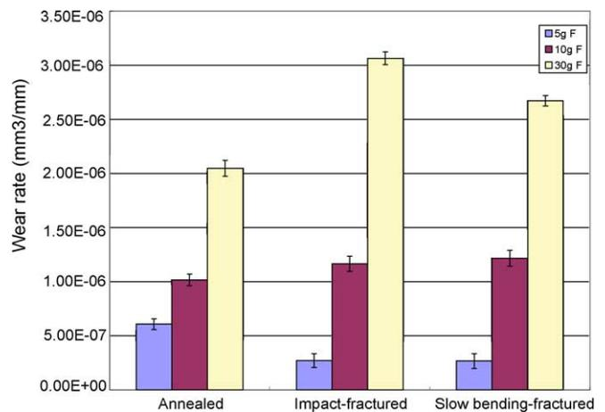
Fig. 11. Wear rates of annealed, impact-fractured, slow bending-fractured surfaces caused by scratch in the 3.5% NaCl solution.
