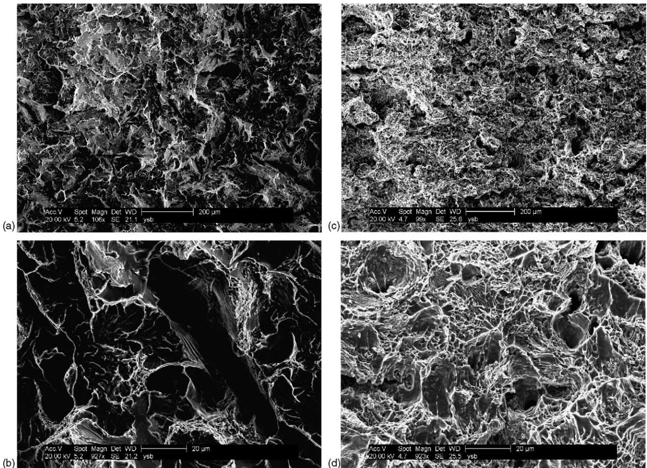
Fig. 2. SEM fracture surface morphology: (a) charpy impact fracture surface; (b) a closer view of the Charpy impact fracture surface; (c) slow bending fracture surface; (d) a closer view of the slow bending fracture surface.
