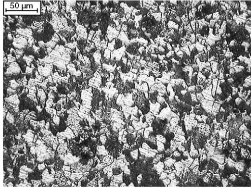
Fig. 1. Optical microstructure of the full-annealed 1045 steel.
