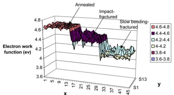
Fig. 9. Electron work functions of full-annealed, impact-fractured and slow bending-fractured surfaces.
