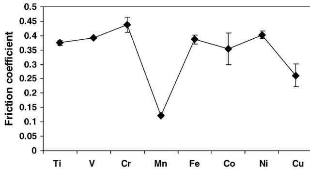
Fig. 1. Friction coefficients of 3d transition metals in contact with iron (under 30 mN).
