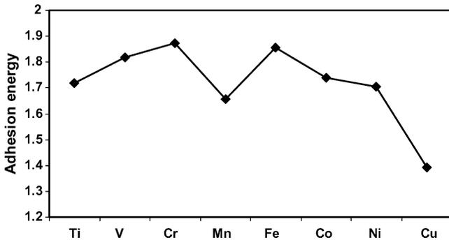
Fig. 4. Adhesion energy (dimensionless) for 3d transition metals in contact with Fe calculated using Eqs. (1) and (5).
