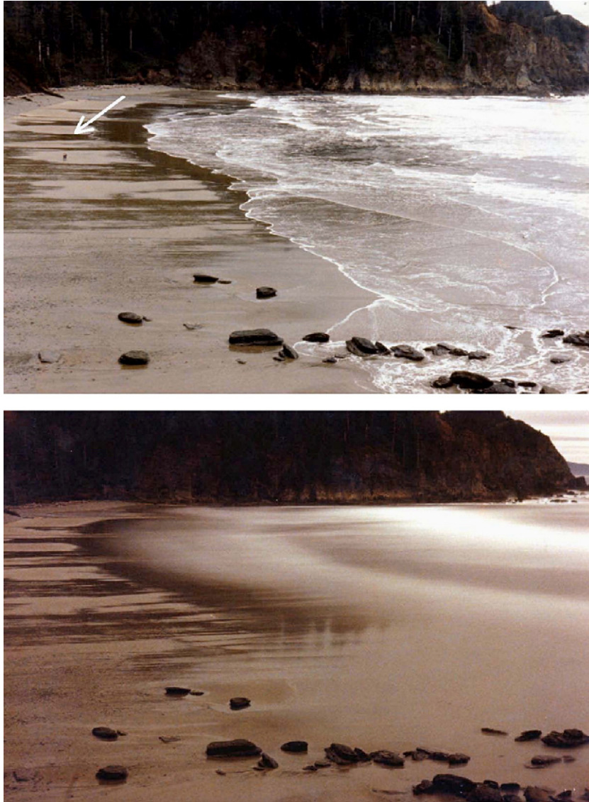
Fig. 2. Example snapshot (upper) and time-exposure (lower) image pair. While hourly collection of these images is now routine, this time-exposure image happens to be the first used for nearshore studies and was taken photographically in 1982 at Short Sands Beach, Oregon. The objective was to find longshore nodes of runup associated with standing edge waves, trapped in this 800 m long pocket beach. While unsuccessful, the accidental discovery of a white band offshore associated with (and indicative of) preferential breaking over a submerged sand bar formed the basis for the eventual development of Argus Stations. The white arrow in the upper image indicates two people conveniently walking along the beach to provide scale.
