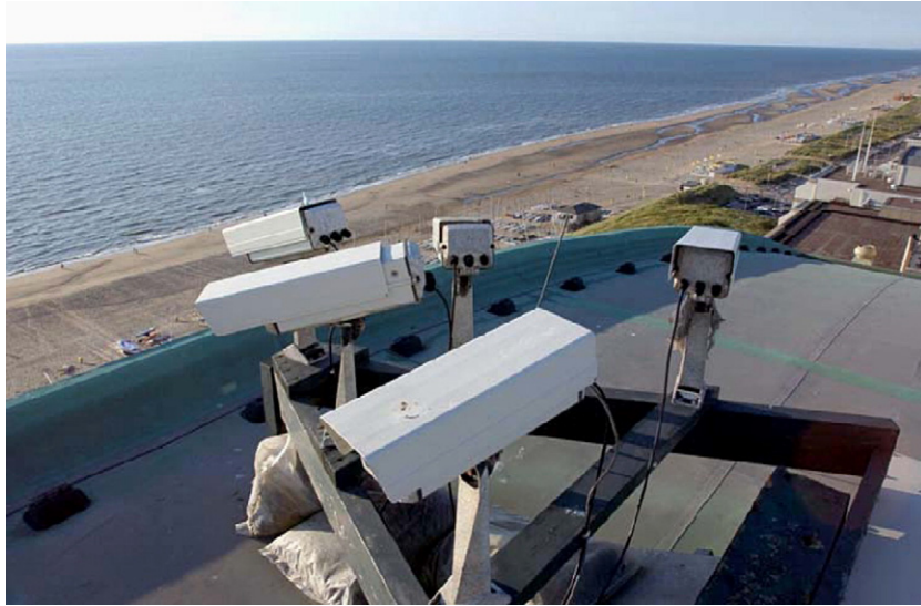
Fig. 1. Camera configuration for the Noordwijk Argus Station in The Netherlands. Argus Stations consist of a suite of cameras rigidly mounted on a roof or tower, and a computer with communications link to the world for control and data return, plus a timing module to synchronize collections between the cameras. Sites also require survey Ground Control Points in the field of view of each camera to allow estimation of the geometry of each view.
