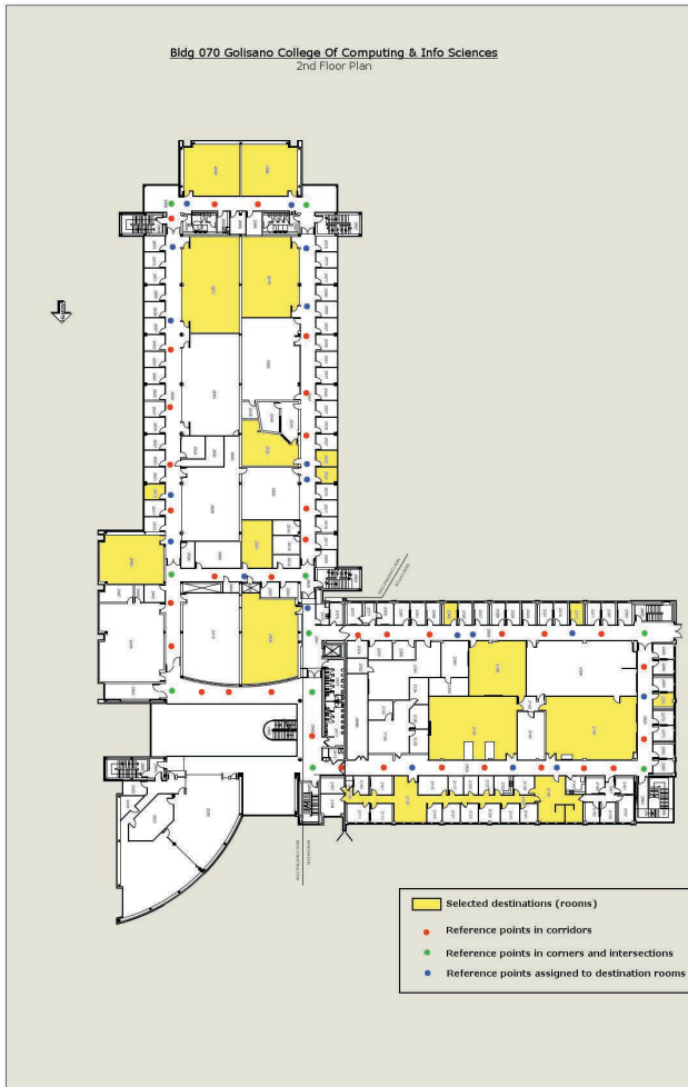
Figure 3: The map of the work area with the selected reference points (fingerprints). The distance between each two adjacent points is 2.4 meters. Each blue dot in the map represents a destination room and it is located in front of the door of that room.
